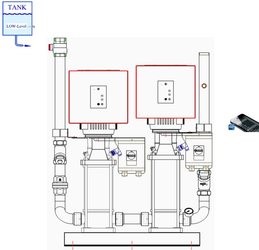
PumpSet FreQ. 38bar 270L/min. Transmitter. TANK supply.
